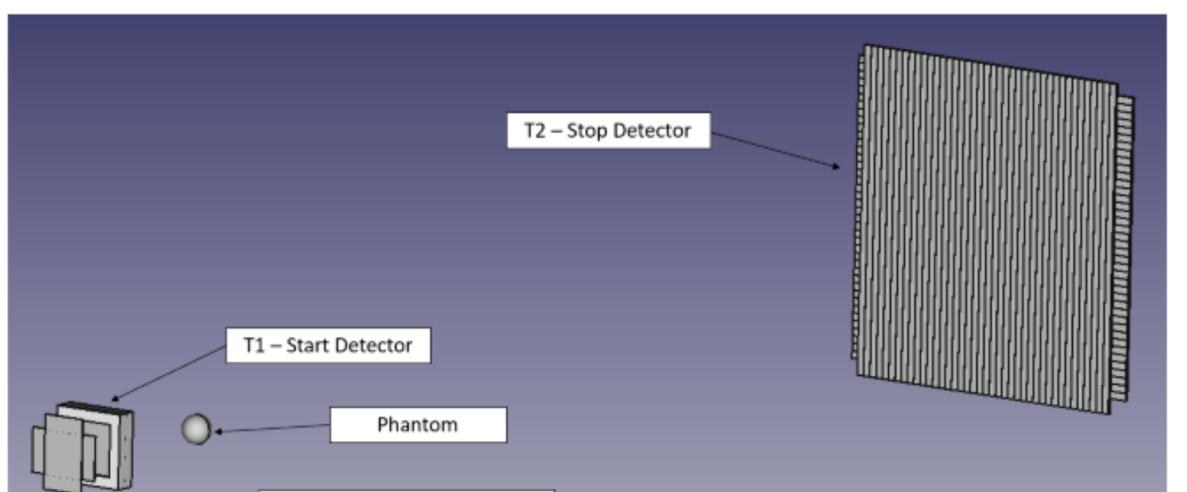
The TOFpRad project aims to assess the viability of a proton radiography system based on the TOF approach by realising a prototype consisting of two fast plastic scintillator detectors for the TOF measurement and a set of layers of plastic scintillator fibres for tracking purposes, both read with SiPMs.
