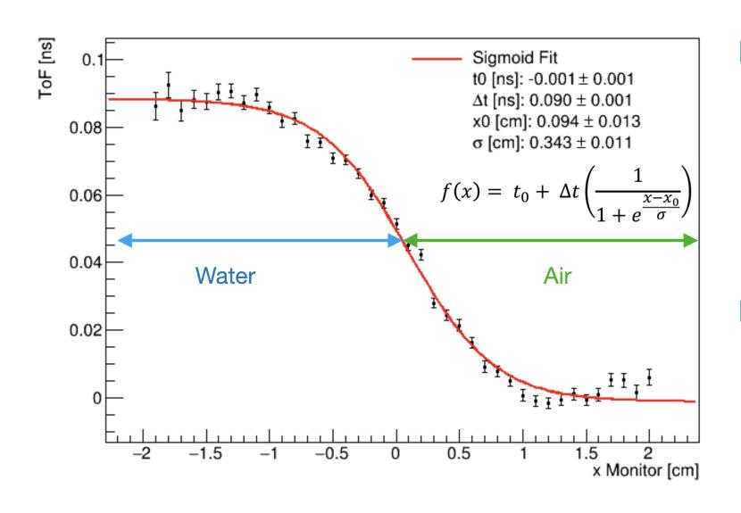
The TOF measurement system has been calibrated varying the beam energy and using a full water equivalent phantom without any air gap
