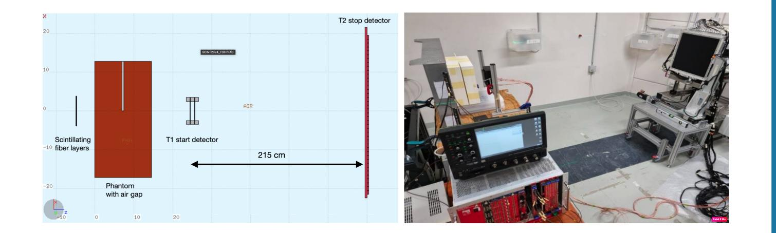
MC simulation by means of FLUKA (left) and picture (right) of the TOFpRad project preliminary experimental setup tested at CNAO.
