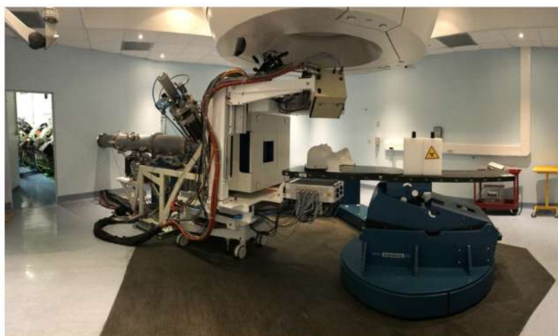
Figure 2.11: View of the treatment room n.1 at CNAO where the INSIDE system is integrated: DP is the beige box and the two PET heads are the white boxes above and below the bed.
