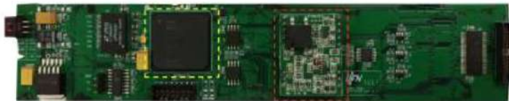
Figure 2.6: Board with FPGA (yellow) and SiPM power supply module (red) highlighted.
