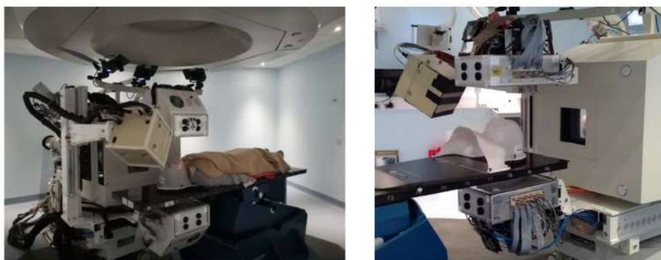
Figure 2.12: View of the INSIDE cart with the DP and the PET heads installed in treatment room n. 1 at CNAO: (left) View of the first patient treated with ^{12}\text{C} ions and monitored with DP. The image also shows the 0° position of the bed. (right) Patient mask attached to the bed to show the position of the DP during a field at 270°.
