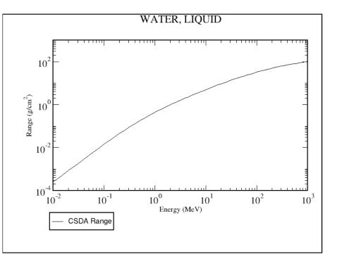
Transport threshold at 1 MeV?  $\rightarrow$  1-MeV e<sup>-r</sup>ange is O(1 mm) = 1000  $\mu$ m Depositing/killing them on the spot in a ~50  $\mu$ m geometry is asking too much...
