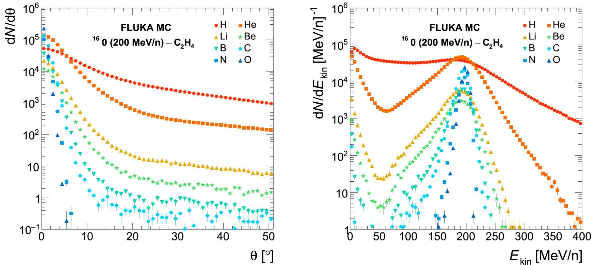
**FIGURE 1** | MC calculation [33, 34] of the angular (**Left**) and kinetic energy (**Right**) distributions of different fragments produced by a 200 MeV/nucleon  $^{16}\text{O}$  beam impinging on a  $\text{C}_2\text{H}_4$  target.
